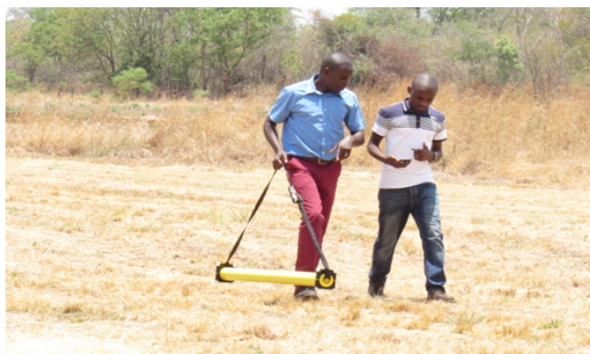
A Dualem-1 geophysical survey instrument (yellow) being carried and used for field data collection.
