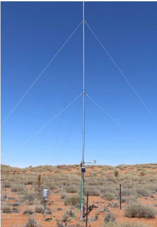
Figure 6: Example of a SASSCAL Automatic Weather
