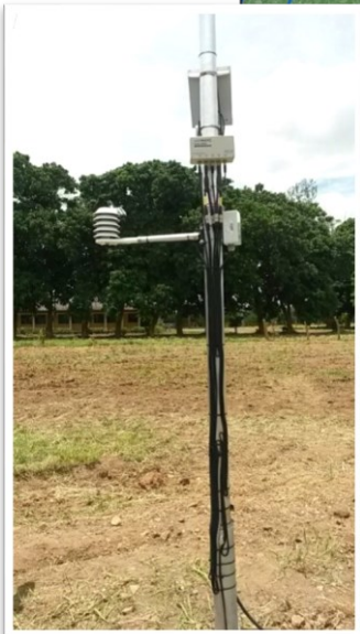
(bottom) The AWS at in Kalamo and (right) SASSCAL WeatherNet AWS in Zambia
